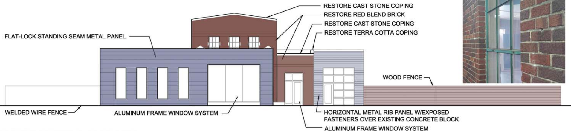
① EAST WASHINGTON AVENUE ELEVATION (SOUTH) 1/8"=1'-0"
